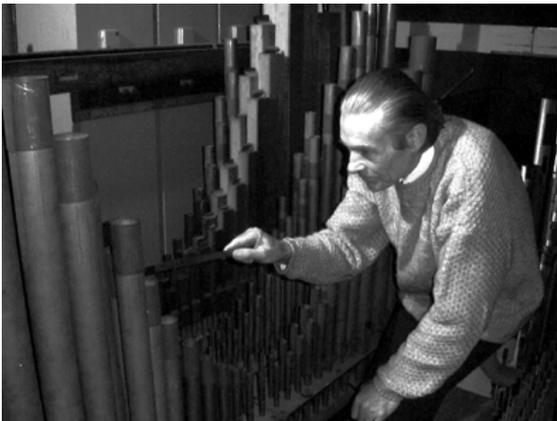
Richard Moth tuning the F# pipe in the open diapason register behind the main organ pipes in the organ loft.
